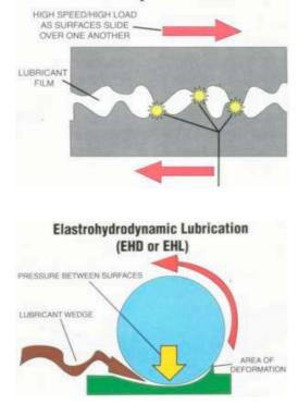
**Boundary Lubrication** is a condition in which the lubricant film becomes too thin to provide total surface separation. This may be due to excessive loading, low speeds or a change in the fluid's characteristics. In such a case, contact between surface asperities (or peaks and valleys) occurs. Friction reduction and wear protection is then provided via chemical compounds rather than through properties of the lubricating fluid.
